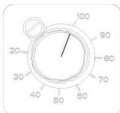
Fig. 9.2 Setting of the metering output (mechanical)
