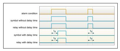
Image 5 Unlatched limit contact without acknowledgment option
