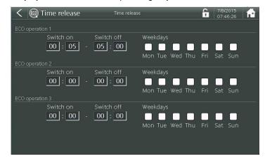
If you select both functions "ECO Timer" and "Circulation," both conditions must be met for the 700 P electronics module to switch to "ECO Mode." If the "DIN function" is selected in the "DIN/ECO function" settings menu, all DIN conditions must be met additionally for switching to ECO mode.
