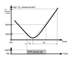
The adaption programme automatically determines the control parameters for free chlorine during commissioning. The adaption can be run separately for normal operation and ECO mode in order to find the suitable controller parameters for both operating modes.
