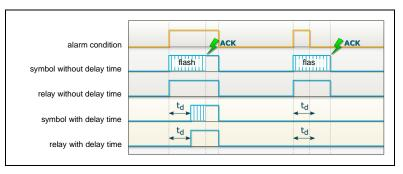
Image 7 Latched alarm with acknowledgment (acknowledgment option)
