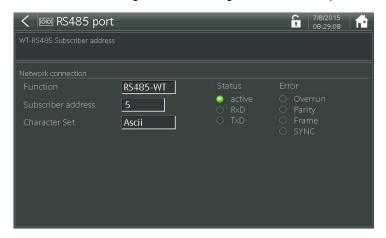
The RS485 interface function can be selected via the input field "Function." To do this, tap the input field. Selection options are displayed. If Fieldbus is selected and a Fieldbus gateway is connected to the RS485 interface, various menus are shown, depending on the gateway.
