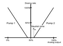
Output behaviour is similar to "Analog output controller (2-point)", but with 50 % offset. This means that with a control deviation of 0 % (setpoint = actual value) a current of 10 mA or 12 mA is output (pump is idle).
