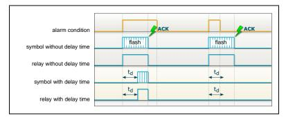
Image 6 Latched alarm with reset acknowledgment option
