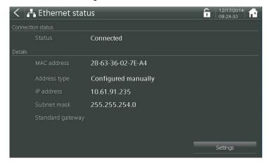
This screen shows the connection status, MAC address of the unit and the IP address settings.
