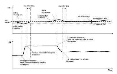
Image 4 Operating principle of the CEDOX operating mode
