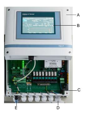
Image 2 700 P electronics module with open cover
