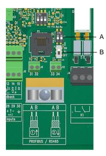
The RS485 interface is used for data transfer to superordinate guide systems such as Process Monitoring system or other systems that support the Wallace & Tiernan RS485 protocol. For more detailed information, please refer to the instruction manual "RS485 interface". These can be requested from your affiliate or download from our website.
