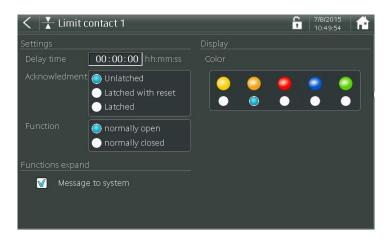
**6** Press the "Relay" button, then you can assign relays to the limit contacts.
