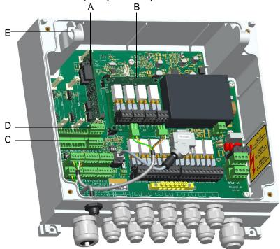
Image 1 Cross-section of 700 P electronics module
