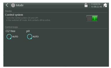
**3** The control system can be switched on or off.To do so, press the button and select (I/O).
