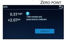
2 Press the desired calibration selection. The example here shows chlorine zero point calibration. A further screen opens with information describing the calibration process.
