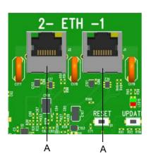
The Blu-Sentinel SE has two integrated Ethernet interfaces (ETH 1 and ETH 2). They are connected internally via an Ethernet switch. The MAC address is displayed in the menu "Information". The installed LAN interface allows data visualization via Internet-capable devices and HTTP protocol or standard browser. The LAN interface also supports data communication via the Modbus TCP protocol, see Chapter 4.4 "Modbus TCP interface".
