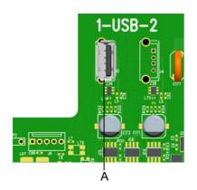
The electronics module is equipped internally with a USB interface. It is used to update the firmware via USB stick (see Chapter 6.5 "Firmware update") or for use as a data logger via USB stick. If a memory stick (W2T866279) is permanently installed in the USB port, monthly archive files are saved in CSV format. All measurements, controller outputs and states of the digital inputs are saved every two minutes.
