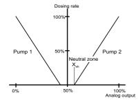
Pump 1 decreases the control value, Pump 2 increases the control value.
