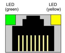
The Ethernet connection is designed in accordance with IEEE 802.3. There are two I8P8C sockets (often referred to as RJ45 sockets) installed. Connection to the HUB or switch can be realized with a 1:1-wire and screened patch cable. Direct connection to a PC network card is possible using a patch cable (1:1) or a crossover cable (crossed network cable). The LEDs are fitted in the 8P8C socket. They display the interface statuses. The meaning of the LEDS is as follows:
