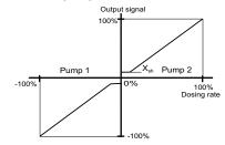
Pump 1 decreases the control value, Pump 2 increases the control value.
