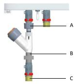
Fig. 3 Section, installation of strainer
