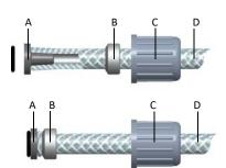
Fig. 5 Detail of hose screw connection
