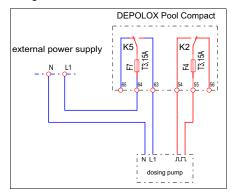
Fig. 10 Plan of terminal assignment
