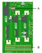
Fig. 2 Detail of PCB - RS485 interface
