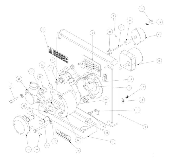
MICRO/2000® AND DEOX/2000® WETSIDE CASTING ASSEMBLY - PARTS — W3T140748 (240V) W3T332446 (115V)
