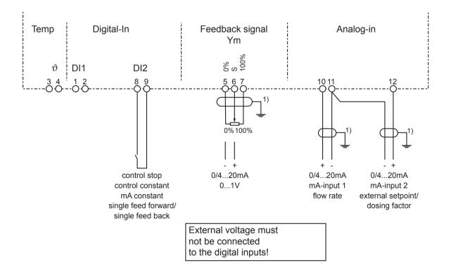
SFC - SCHEMATIC WIRING
