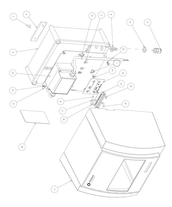
MICRO/2000® AND DEOX/2000® CE WETSIDE ENCLOSURE ASSEMBLY - PARTS — W3T140748 (240V) W3T332446 (115V)
