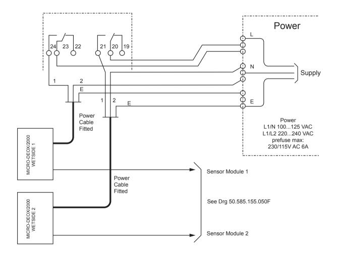
Relay Outputs - MICRO/2000 - DEOX/2000 Wet Side Power Connection
