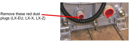
Figure 3-1b LX-EU, LX-X, LX-Z modules (BSPM) with red shipping plugs
