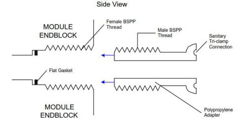
Figure 3-4 LX Piping Adapter Sealing Mechanism: HWS Modules
