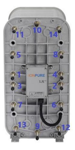
Figure 3-2 LX Tightening Sequence
