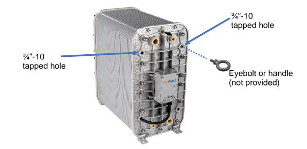
Figure 1-2: LX Module Lifting Points (Cathode/Plumbing Side Shown)
