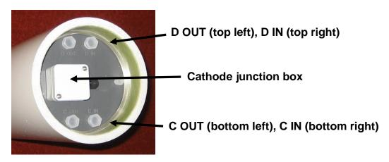
Figure 3-1: MX plumbing connections – cathode end
