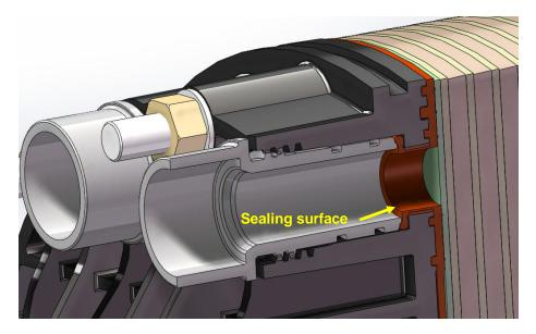
**USE OF SEALANTS** - DO NOT use Teflon® tape or any other pipe sealant (such as pipe dope) on the VNX ACME thread adapters. The use of these products on the VNX adapters will prevent good sealing.
