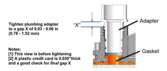
Figure 3-4 Proper Tightening of VNX Piping Adapter
