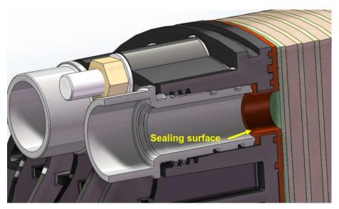
Figure 3-3 VNX Piping Adapter Sealing Mechanism
