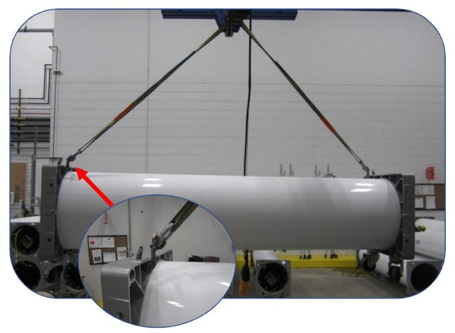
Figure 2-1 Lifting VNX module via housing FlexMounts
