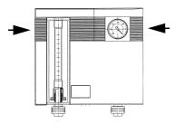
1 Hold the cover at both sides, press your thumb on the manometer and pull away the cover at both sides at the same time.
