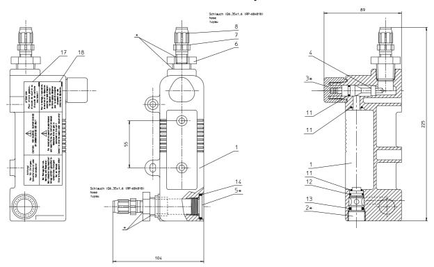
\* slightly grease and tighten the thread with special grease W3T165077
