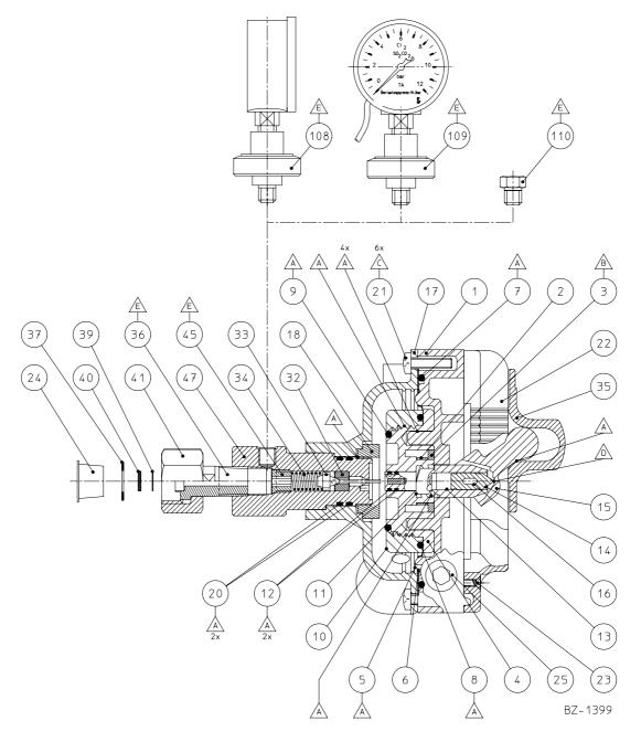
A, D: Before assembly: Slightly grease with special grease W3T165077
