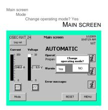
When performing maintenance work or to shut the system down for a short period, switch off automatic mode.
