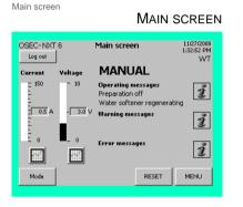
The chlorine membrane electrolysis system is in the "Preparation off" operating state. The system is ready to operate.
