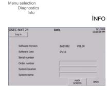
3 Switch to the "Info" screen. If necessary, enter further details about the chlorine membrane electrolysis system in the "Order number", "System location" and "System name" input boxes. You will be asked to enter a username and password. For details, see chapter 5.2.2 Logging in.
