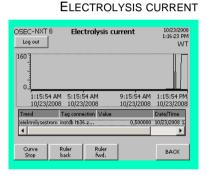
The two buttons below the bar can be used to display the course of the electrolysis current and the cell voltage over the past 12 hours for diagnostic purposes.
