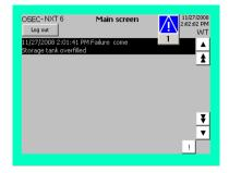
If the system develops a fault, a corresponding error message is displayed, irrespective of the current operating state or what else is currently being displayed by the system. Every error message has to be acknowledged individually by pressing the i button. Once the last error message has been acknowledged the display returns to the last menu that was displayed and the symbol is displayed.
