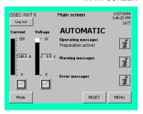
If the chlorine membrane electrolysis system is in the "Preparation active!" operating state, it begins the run-up process ("Preparation run-up"). The "Preparation active!" operating state has three phases:
