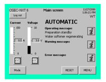
Automatic regeneration is active throughout the preparation process. If regeneration starts, the preparation process is interrupted, the system switches to run-out or stops run-out and remains in the "Preparation standby" state. Regeneration is running. This is indicated on the display. Once regeneration has finished, sodium hypochlorite preparation automatically starts again as soon as the "Storage tank min." fill level in the storage tank is reached.
