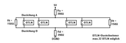
Both ends of the bus cable must be connected to a moving load Rt (150 Ohm). Symmetry is assured at only one point of the bus.
