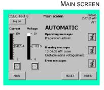
If the power supply fails (see chapter Installation, 4.5.1 Checking the power supply), the warning "Unstable mains voltage/mains failure" is displayed.
