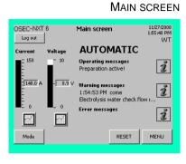
If the actual electrolysis water flow rate differs from the setpoint (see the signs on the chlorine membrane electrolysis system), the warning "Electrolysis water check flow rate" is displayed.
