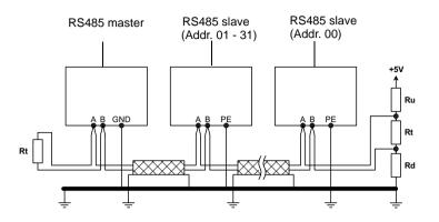
The earth bus or earth electrode conductor  $>= 6 \text{ mm}^2$  must be laid parallel to the bus cable.
