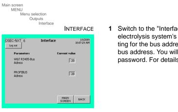
1 Switch to the "Interface" screen on the chlorine membrane electrolysis system's control and display unit. The factory setting for the bus addresses is 20. If necessary change the Profibus address. You will be asked to enter a username and password. For details, see chapter 5.2.2 Logging in.
