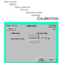
3 The flow rate can be adjusted by pressing "+" or "-" in the "Calibration" submenu if necessary.
