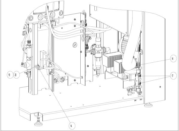
Bild 2 Wear parts to be replaced
