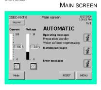
Automatic regeneration is usage-based and depends on the water hardness. The automatic regeneration of the water softener is active in every operating state. If regeneration is running, this is indicated on the display. Press the "i" (Info) button to show the current regeneration phase:
