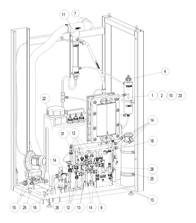
Bild 1 Wear parts to be replaced
