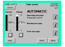
If the level in the sodium hypochlorite storage tank is below "Storage tank min." the chlorine membrane electrolysis system will switch to the "Preparation active" state.
