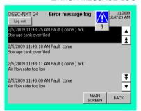
All of the error messages are are stored in the "Error message log" together with the date, time and status details ("come" and "gone") and can be viewed at any time. See chapter 5.12.3 Error message log for details.
