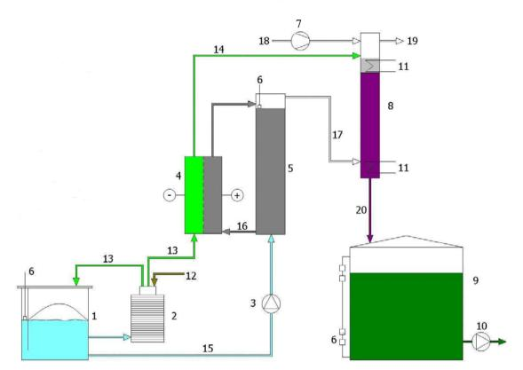
Fig. 1 Chlorine membrane electrolysis system
