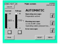
If the actual operating water pressure exceeds the setpoint (see the information label on the chlorine membrane electrolysis system) the warning "Operating water pressure too high" is displayed.
