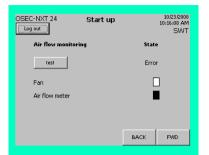
The test takes between 30 seconds and 6 minutes at most. If there is an error once the time limit has been reached, the message "Error" is displayed.
