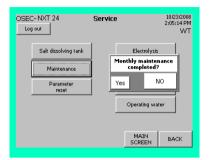
Regular service of the chlorine membrane electrolysis system is part of the liability for defects. There are certain tasks that the operator is required to perform on a daily, weekly or monthly basis. Once a year, annual maintenance must be carried out by Evoqua service personnel or by personnel trained and authorized by Evoqua for maintenance work. When monthly or annual maintenance is due a warning message is displayed on the main screen.
