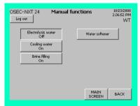
Electrolysis water can be turned on manually either for diagnostic purposes or when performing maintenance, for instance to set the flow rate or to calibrate the electrolysis water flow meter.
