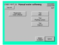
Automatic regeneration of the water softener is usage-based and depends on the water hardness. Regeneration of the water softener can also be started manually.
