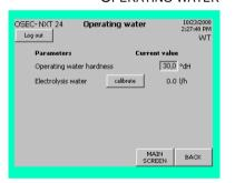
2 Switch to the "Operating water" menu. This is where the current electrolysis water flow rate is displayed. If it differs by more than +/- 0.5 l/h from the system-specific setting on the dosing ball valve, press the "calibrate" button. You will be asked to enter a user name and password. For details, see chapter 5.2.2 Logging in.
