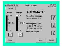
Once the fill level in the storage tank reaches the "Storage tank empty" level, the warning message "Storage tank empty" is displayed.
