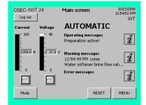
If the actual brine flow rate in the water softener differs from the setpoint the warning "Water softener check brine flow" is displayed.
