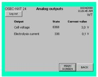
In the "Analog outputs" menu service personnel can view the current values and states of the analog outputs for the cell voltage and the electrolysis current for diagnostic purposes.
