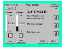
If both of these conditions are met the "Start preparation" button is also displayed on the basic display.
