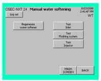
Testing the water softener water inlet solenoid valve (E5).
