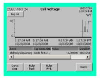
The two buttons below the bar can be used to display the course of the electrolysis current and the cell voltage over the past 12 hours for diagnostic purposes.
