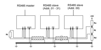
The earth bus or earth electrode conductor >= 6 mm<sup>2</sup> must be laid parallel to the bus cable.
