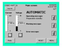
Once electrolysis power is reached, the chlorine membrane electrolysis system switches to the product preparation state and prepares sodium hypochlorite until the "Storage tank max." level is reached in the sodium hypochlorite storage tank. Then the system remains in the "Preparation standby" state. For details see chapter Operation, 5.3 Automatic operation.
