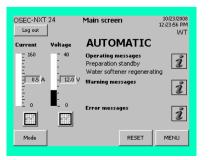
Once electrolysis power is reached, the chlorine membrane electrolysis system switches to the product preparation state and prepares sodium hypochlorite until the "Storage tank max." level is reached in the storage tank.
