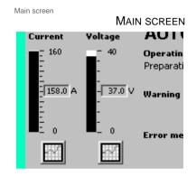
The current cell voltage and electrolysis current can be seen on the main screen at all times. They are displayed both as a bar and as a number to the right of the bar.
