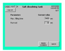
The "Salt dissolving tank" menu is used to enter limits for the max. filling time and run-out time for the salt dissolving tank. If the values entered here are exceeded an error message is generated.
