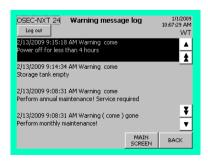
The "i" (Info) button allows you to view the current warning messages that have been displayed by the system, including the date, time and status details ("come"), at any time.
