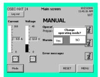
The chlorine membrane electrolysis system is running in automatic mode. Automatic preparation is turned on and off by pressing the "Mode" button (see chapters 5.6 Activating manual preparation and chapter 5.7 Stopping preparation manually for details). The display shows if automatic mode is active.
