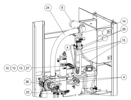
Fig. 2 Wear parts to be replaced
