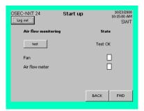
Check that the air flow monitor is working correctly when the fan is off. If air is not flowing, the status indicator changes from black to white. This means that the air flow monitor is working correctly, and the message "Test OK" is displayed.
