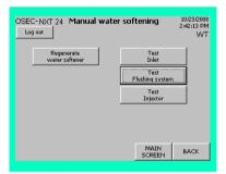
Testing the water softener flushing solenoid valve (E8).
