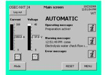
If the actual electrolysis water flow rate differs from the setpoint (see the sign on the chlorine membrane electrolysis system), the warning "Electrolysis water check flow rate" is displayed.
