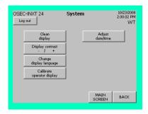
IIn the "System" menu you can configure the control and display unit.
