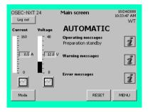
The chlorine membrane electrolysis system is now in automatic preparation mode. If automatic mode is active, this is shown on the display as a text message. For details, see chapter 5.3 Automatic mode and chapter 5.8 Operating messages.
