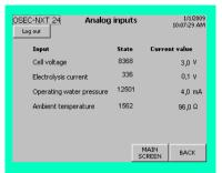
In the "Analog inputs" menu service personnel can view the current values and states of the analog inputs for the cell voltage and the electrolysis current, the operating water pressure and the ambient temperature for diagnostic purposes.
