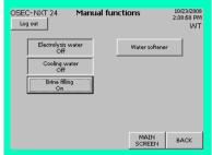
The brine pump can be turned on manually, either for diagnostic purposes or when performing maintenance.
