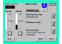
The chlorine membrane electrolysis system is in the "Preparation off" operating state. The system is ready to operate.
