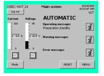
Once the run-out process has been completed, the system reverts to the "Preparation standby" operating state.
