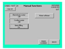
23 Refill the anode chamber with brine immediately. Switch to the "Manual functions" screen and press the "Brine filling On" button. When the fluid level limit is reached in the chlorine separator the brine pump stops automatically. The manual brine pump function is simultaneously turned off.
