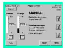
The chlorine membrane electrolysis system is in "MANUAL" mode in the "Preparation off" operating state. The system is now ready to operate.
