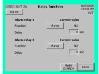
Both of the alarm relays, 1 and 2, require an NC (normally closed) or NO (normally open) switching function. If a time delay is needed before the switching function is triggered, you can also specify a delay of between 0 and 3600 seconds.
