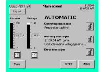
If the power supply fails (see chapter Installation, 4.5.1 Checking the power supply), the warning "Unstable mains voltage/mains failure" is displayed.
