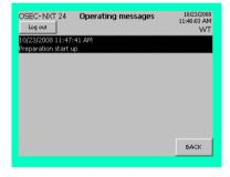
Once the "Storage tank min." fill level in the storage tank is reached, the level switch automatically starts sodium hypochlorite preparation again. The system then switches to the run-up phase of the "Preparation active!" operating state.
