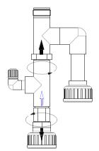
Fig. 4 Dismantle injector
