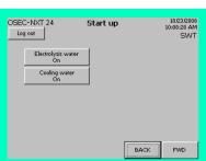
2 To confirm that you wish to shut the system down, press "Yes". The display then switches to the start-up menu and the system can be switched off at the main switch.
