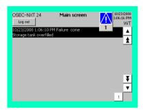
If the system develops a fault, a corresponding error message is displayed, irrespective of the current operating state or what else is currently being displayed by the system. Every error message has to be acknowledged individually by pressing the \_\_\_\_ button. Once the last error message has been acknowledged the display returns to the last menu that was displayed and the \_\_\_\_ symbol is displayed.
