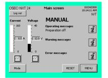
If the chlorine membrane electrolysis system is in the "Preparation active!" operating state, it first goes through the run-out process before then switching automatic mode off.
