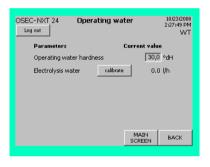
The "Operating water" menu is used to enter the total operating water hardness (factory default 30° dH) and to calibrate the flow meter for the electrolysis water, if necessary. You will be asked to enter a user name and password. For details, see chapter 5.2.2 Logging in.
