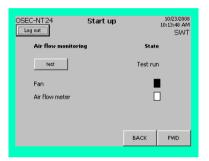
3 Press the "test" button to check that the air flow monitor is working correctly. The fan starts turning and the corresponding status indicator changes from white to black.
