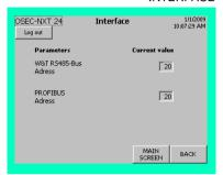
1 Switch to the "Interface" screen on the chlorine membrane electrolysis system's control and display unit. The factory setting for the bus addresses is 20. If necessary change the PROFIBUS address. You will be asked to enter a username and password. For details, see chapter 5.2.2 Logging in.
