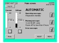
The chlorine membrane electrolysis system is capable of displaying twelve different warning messages. The last warning message reported by the system is displayed as a text message on the main screen, together with the time stamp and the state and the "i" (Info) button flashes:
