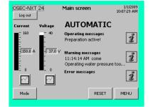
If the actual operating water pressure drops below the setpoint (see the information label on the chlorine membrane electrolysis system) the warning "Operating water pressure too low" is displayed.
