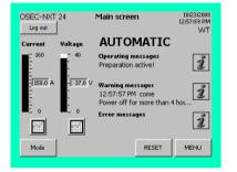
If there is a power failure lasting more than 4 hours, the warning "Power off for more than 4 hours" is displayed for 10 seconds.
