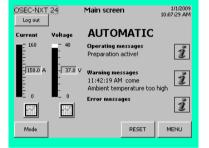
If the actual ambient temperature exceeds the set limit the warning "Ambient temperature too high" is displayed.
