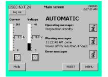
If there is a short power failure (< 4 h) the warning "Power off for less than 4 hours" is displayed for 10 seconds.
