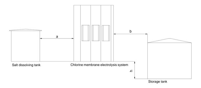
Fig. 1 Setup of the chlorine membrane electrolysis with accessories, permissible distances
