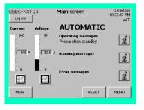
In automatic mode, sodium hypochlorite preparation is controlled via the level switch in the storage tank. The system is initially in the operating state "Preparation standby". Once the "Storage tank min." level is reached, sodium hypochlorite preparation begins.
