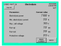
The "Electrolysis" menu is used to set all of the key parameters for the electrolysis process. These settings are configured at the factory and are system-specific. They are therefore password protected and only accessible to level 3 service personnel.
