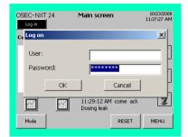
4 Press OK to confirm. The display then returns to the previous menu and the "Log in" button changes into a "Log out" button. The required functions are now accessible.
