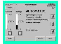
Automatic regeneration is usage-based and depends on the water hardness. The automatic regeneration of the water softener is active in every operating state. If regeneration is running, this is indicated on the display. Press the "i" (Info) button to show the current regeneration phase:
