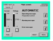
If the chlorine membrane electrolysis system is in the "Preparation active!" operating state, it begins the run-up process (Preparation start up). The "Preparation active!" operating state has three phases:
