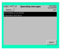
The chlorine membrane electrolysis system then switches to the run-out phase ("Preparation shut down").
