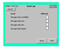
If the level switches are correctly adjusted and the storage tank is empty, the display should appear as shown on the left.
