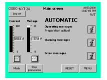
If both of these conditions are met the "Stop preparation" button is also displayed on the main screen.
