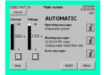
If the actual cooling water flow rate differs from the setpoint (see the sign on the chlorine membrane electrolysis system), the warning "Cooling water check flow rate" is displayed.
