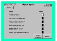
In the "Digital inputs" menu you can view the current status of the digital inputs for diagnostic purposes.
