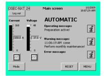
The warning "Perform monthly maintenance!" is displayed once a month. This warning message can be displayed in every operating state. The chlorine membrane electrolysis system remains operational. The warning message is turned off again once you have confirmed that monthly maintenance has been carried out by pressing the "Maintenance" button on the main "Service" menu, see chapter 5.12.4. See chapter 5.13 Maintenance by the operator for further details on carrying out monthly maintenance.
