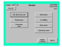
The "Service" menu is primarily intended for use by service personnel (password level 3). All of the settings and operating parameters can, however, be read by all users, in any user group, without requiring the user to log in. From password level 2, the user can enter or change certain system settings.
