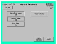
Cooling water can be turned on manually, either for diagnostic purposes or when performing maintenance, for instance to set the flow rate.
