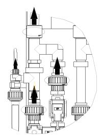
Drain and rinse the chlorine membrane electrolysis system and switch off at the main switch.
