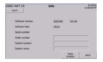
3 Switch to the "Info" screen. If necessary, enter further details about the chlorine membrane electrolysis system in the "Order number", "System location" and "System name" input boxes. You will be asked to enter a username and password. For details, see chapter 5.2.2 Logging in.
