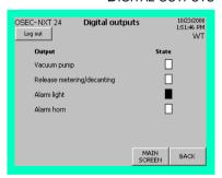
In the "Digital outputs" menu you can view the current status of the digital outputs for diagnostic purposes.
