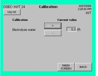
**3** The flow rate can be adjusted by pressing "+" or "-" in the calibration submenu if necessary.
