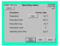
The "Operating data" submenu consists of several screens. Press the "FWD" button to move to the next screen, and "BACK" to go back to the previous screen.
