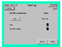
Check that the air flow monitor is working correctly when the fan is on. If air is flowing, the corresponding status indicator changes from white to black.
