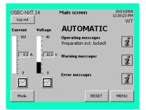
The chlorine membrane electrolysis system control system (available as an option) also provides a digital input for external control of the sodium hypochlorite preparation. This allows the operator to turn off the preparation of sodium hypochlorite from a control room. This is possible in every operating state and is shown on the display.
