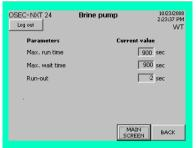
The "Brine pump" menu is used to configure the brine pump. These settings are configured at the factory and are system-specific. They are therefore password protected and only accessible to level 3 service personnel.
