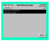
Once the run-up process has been completed, the chlorine membrane electrolysis system switches to the preparation phase ("Preparation running") operating state. Sodium hypochlorite preparation stops once the "Storage tank max." fill level is reached.
