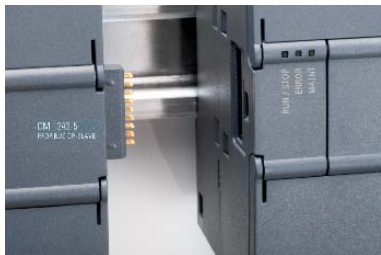
Installing the communication module
