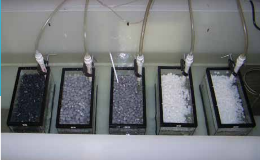
Side-by-side testing validates performance at 800 m 2 /m 3 surface area.
