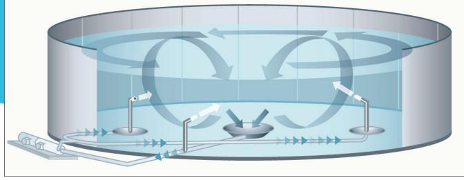
The JetMix™ mixing system creates a very efficient mixing pattern as shown above and demonstrated on the cover graphic.
