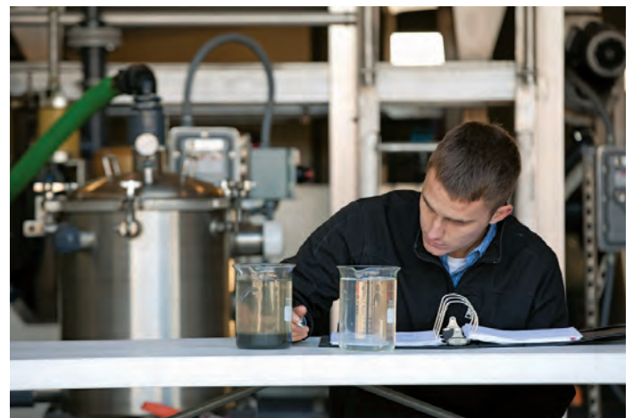
Testing documents the settleability of the mixed liquor suspended solids. The beaker on the left demonstrates the rapid settleability with the BioMag System.
