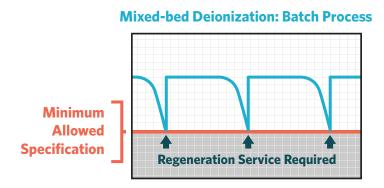
As ion-exchange resins exhaust, contaminants begin to break through, eventually requiring downtime for resin regeneration or replacement.
