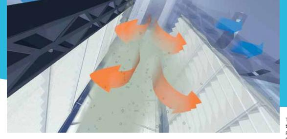
The inside-out flow of the Forty-X<sup>™</sup> disc filter panels effectively captures suspended solids and adds to backwashing efficiency.
