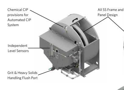
The Forty-X<sup>™</sup> Disc Filter Armor Lite offers a modular design that is flexibility and dependable for municipal and industrial filtration applications. The pre-screen is like "Armor" for the disc filter, providing initial filtration of large organic and inorganic materials.
