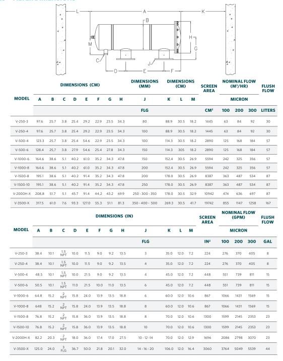
Nominal flow rates shown are the maximum flow rate for that model with 100, 200, and 300 micron screens for demonstration purposes only. Larger micron ratings result in higher allowable flow rates. Smaller micron ratings result in lower allowable flow rates.
