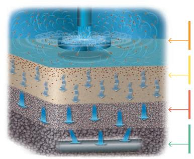
Cross-Flow: VortiJet injector induces a cross-flow pattern across surface of media. Large particles are kept in suspension which prevent media surface blinding.
