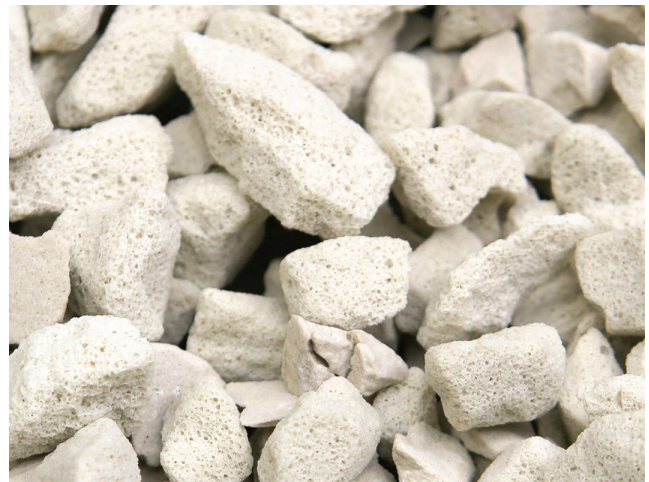
Long-lasting, nondegradable Bioglas® media.
